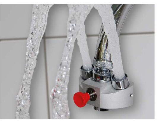
Mini eyewash station ideal for the lab, filling stations or all work places where aggressive substances are used. Eyes Fresh can be attached to any standard cold water tap. For normal use of the tap, just press the button and the function changes back from the eye wash (returns automatically to eyewash-function when the tap is closed). Can be fitted onto taps with M22x1, 1/2" or 3/8" outer thread. With sufficient water pressure provided, performance according to DIN EN 15154-2.
